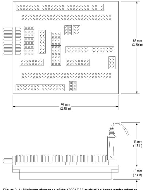
Figure 3–6: Minimum clearance of the 68331/332 evaluation board probe adapter
