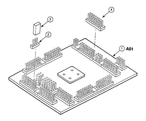
Figure 1: 68331/332 QFP probe adapter exploded view
