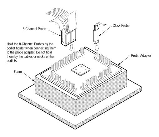
Figure 1-9: Connecting probes to a CQFP probe adapter
