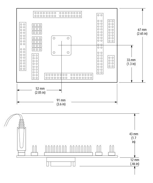
Figure 3-4: Minimum clearance of the 68331/332 QFP probe adapter
