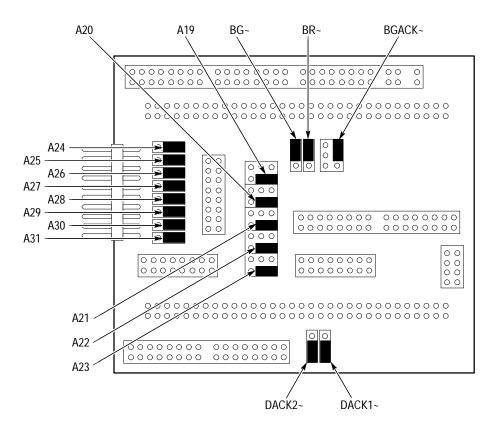
Figure 1–3: Jumper locations on the 68331/332 evaluation board probe adapter
