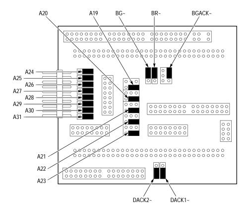
Figure 3–3 shows the location of the jumpers on the 68331/332 Evaluation Board probe adapter.
