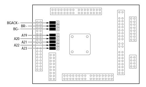
Figure 1–1 shows the location of the jumpers in the default (off) position on the 68331/332 QFP probe adapter.
