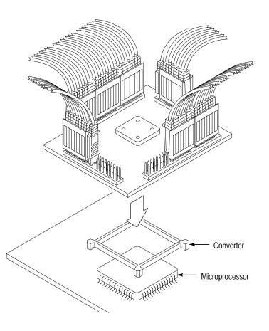
Figure 1–10: Placing a CQFP probe adapter onto the SUT
