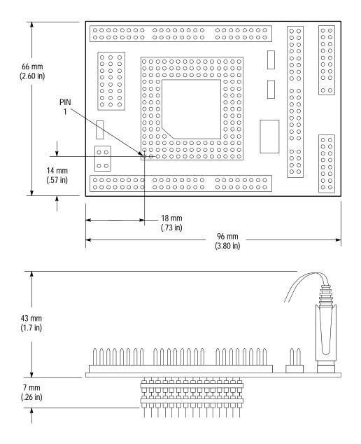
Figure 3–5: Minimum clearance of the 68340 PGA probe adapter
