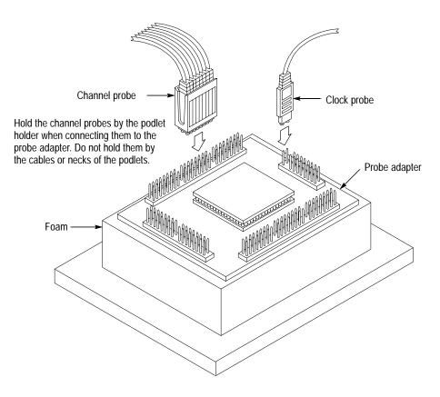
Figure 1–5: Connecting probes to a PGA probe adapter
