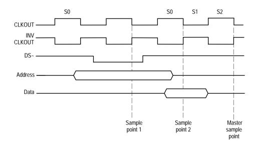
Figure 3–8: CPU32 Family bus timing for a Show Bus cycle
