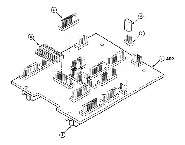
Figure 2: 68331/332 Evaluation Board probe adapter exploded view
