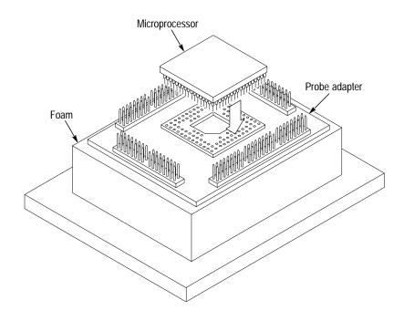
6. Place the microprocessor into the probe adapter as shown in Figure 1–4.
