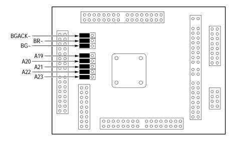
Figure 3–1 shows the location of the jumpers on the 68331/332 QFP probe adapter.
